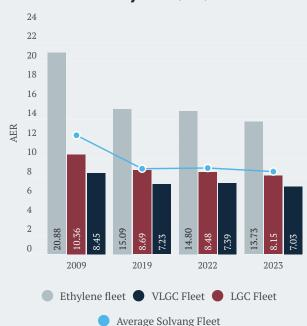
The average AER for the Solvang fleet and for the vessel groups has been recalculated in 2023. By using weighted average for transport work (dead weight \* sailed distance), we get a better picture of the actual AER for the fleet.
